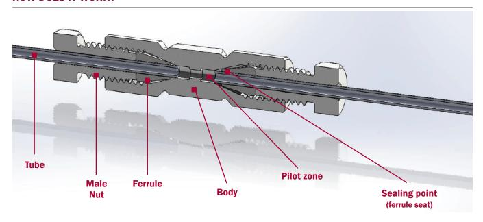
The tube is inserted in a male nut and the ferrule into the body of the fitting until the tube reaches the pilot zone. The tube will not fully penetrate the pilot zone as other types of fittings does.
